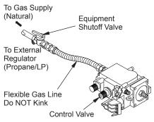
Figure 39 - Connecting Flexible Gas Line to Millivolt Valve
